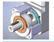
出力軸表面與油封搭配確保最低磨擦係數和減少 啓動負載,保持最佳密封性,延長使用壽命, Grinding process to smooth surface of output shaft, and with oil-seal to minimum friction coefficient and reducing start up load; result in the best seal-ability and extended lifespan.
